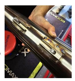
Tighten flange nuts at rear cylinder studs:
